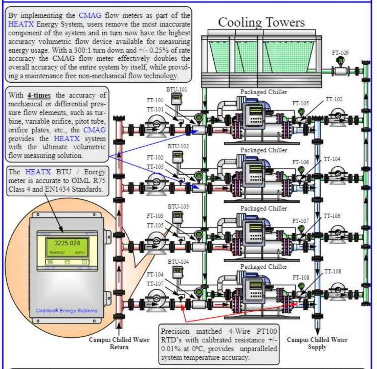
With no moving parts or flow line obstruction the CMAG has no mechanical drift, which require re-calibration, and does not cause system head loss creating an unwanted heat source (for chilled water systems), as do all other mechanical and differential pressure flow technologies typically used.
